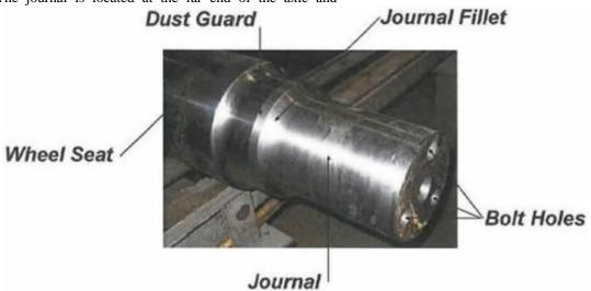
\*707 Railcar axles are made of steel, which has a high stress level and a long life cycle.<sup>2</sup> A pit, crack, nick, dent, or gouge on the fillet or journal of an axle, however, is considered a stress riser. A stress riser is a surface injury or defect that can cause fatigue-induced cracking. The surface injury or defect in this case was corrosion pitting
