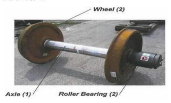
The body of a railcar axle is located between two wheel seats. The wheels sit on the wheel seats, which are located fifteen or sixteen inches from the end of the axle. Beyond each wheel seat, there is a two-inch long dust guard, an inch-and-a-half long fillet, and a journal that measures approximately twelve inches. The wheel seat, dust guard, fillet, and journal comprise the outside end of the axle. The journal is located at the far end of the axle and
